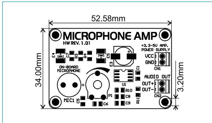
**Figure 3:** Dimensions of the MICROPHONE AMP additional board
