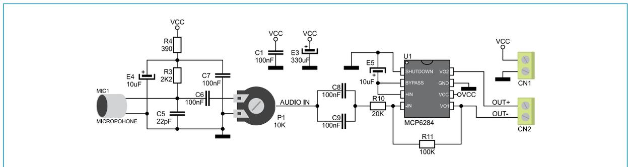
Figure 2: MICROPHONE AMP additional board connection schematic
