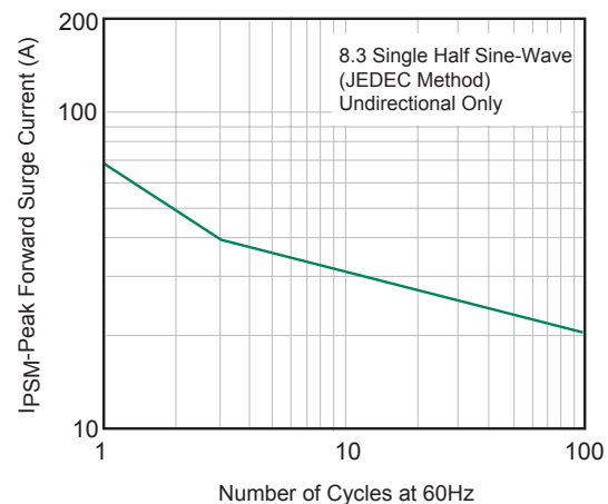
Fig. 6- Maximum Non-Repetitive Forward Surge Current Uni-Directional Only
