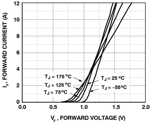
Figure 1. Forward Characteristics
