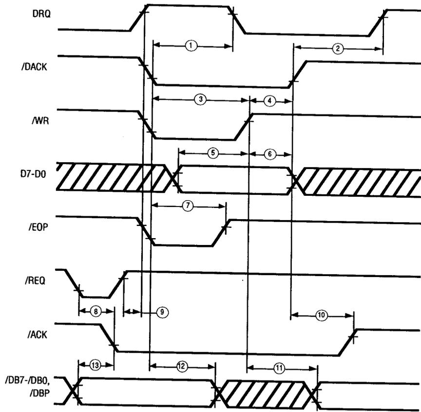
Figure 47. DMA Write (Non-Block Mode) Initiator Send Cycle
