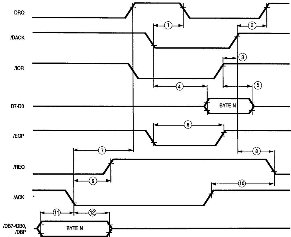
Figure 50. DMA Read (Non-Block Mode) Target Receive
