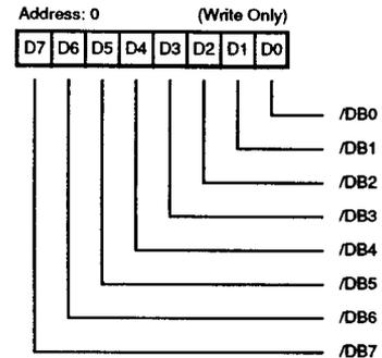
**Figure 6. Output Data Register**
