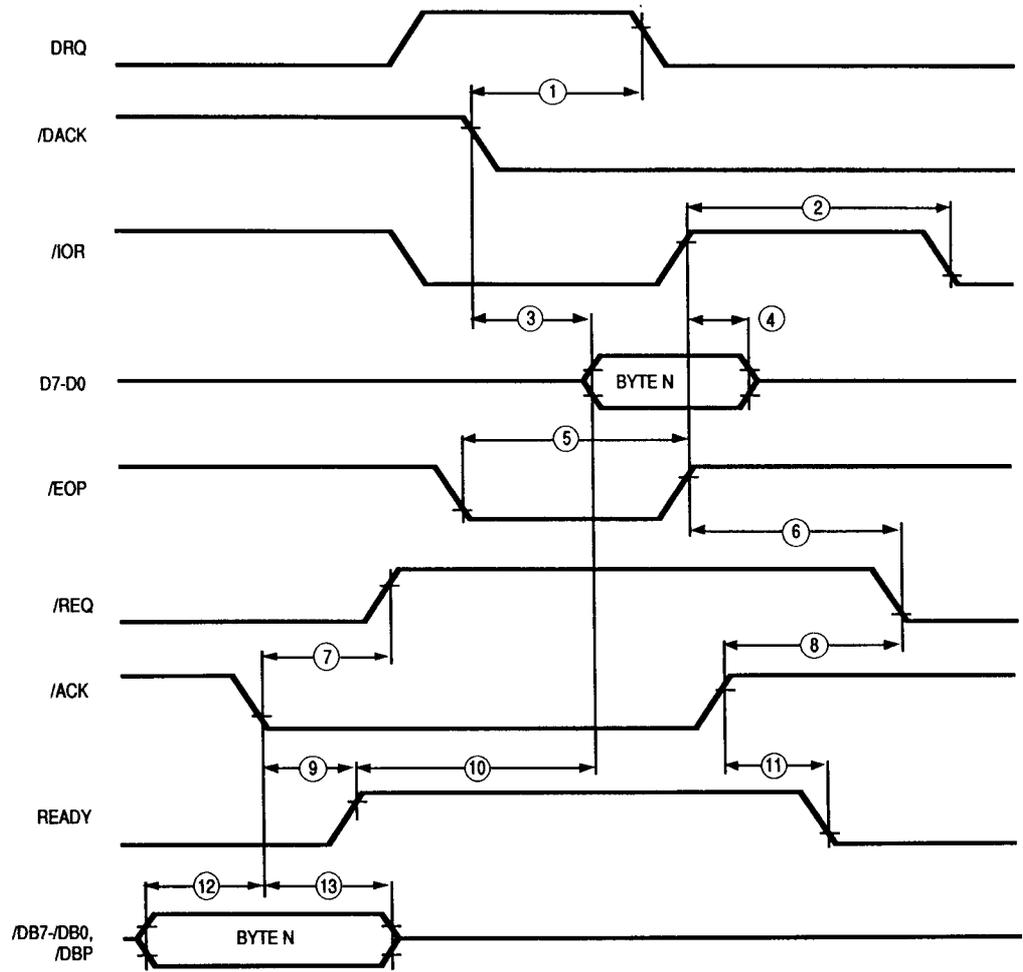
Figure 52. DMA Read (Block Mode) Target Receive
