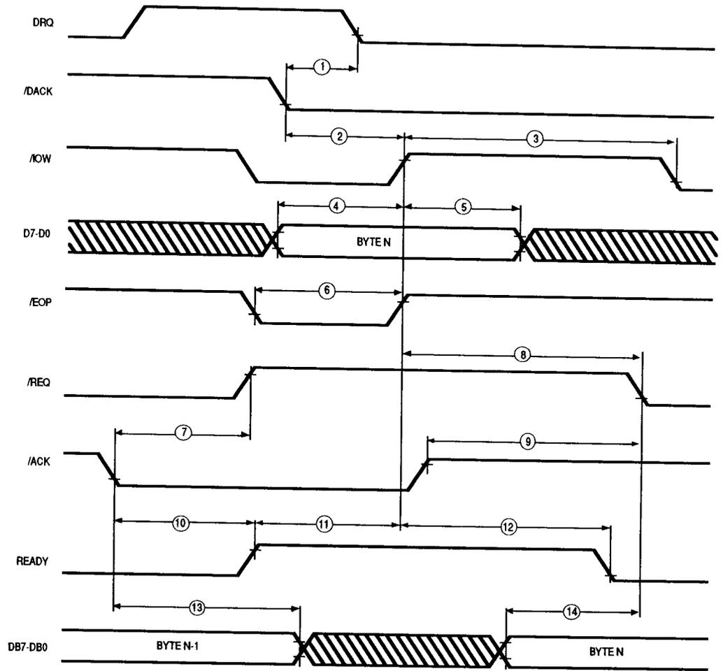
Figure 51. DMA Write (Block Mode) Target Send
