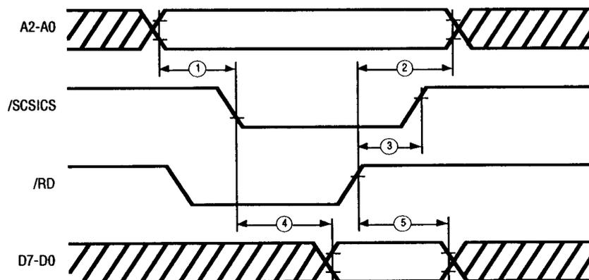
Figure 46. CPU Read Cycle
