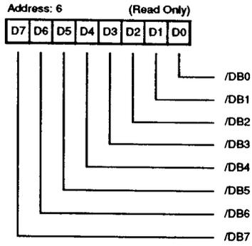
Figure 33. Input Data Register
