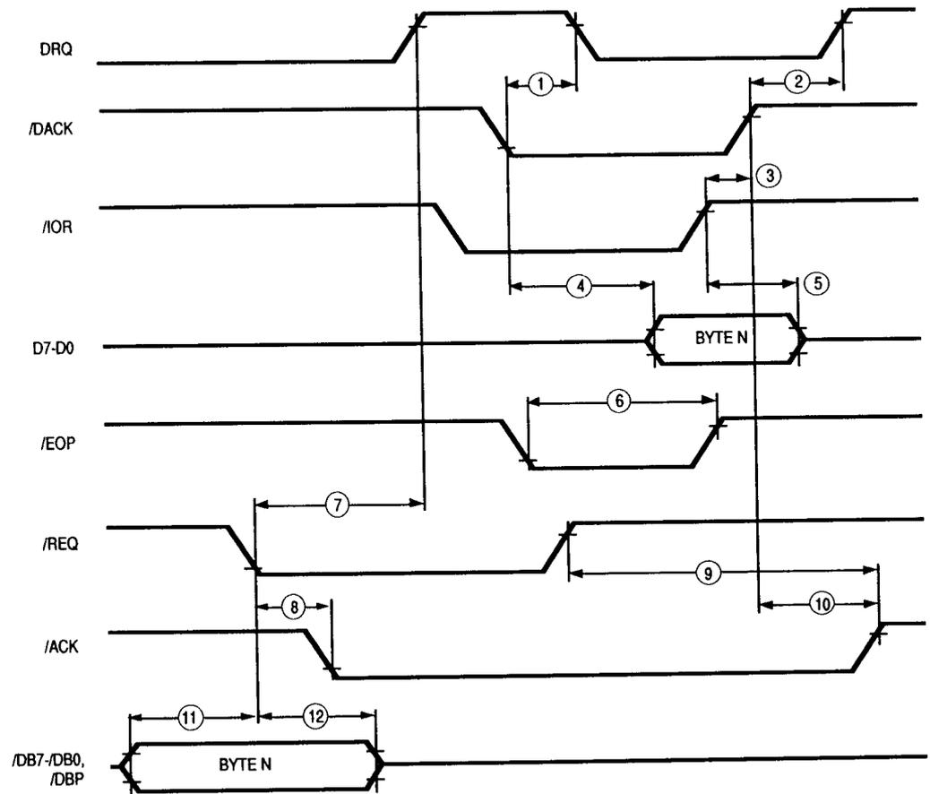
**Figure 48. DMA Read (Non-Block Mode) Initiator Receive**
