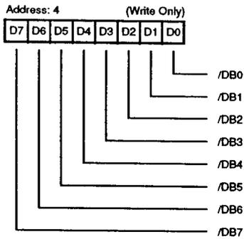
Figure 39. Select Enable Register
