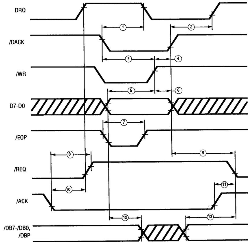
Figure 49. DMA Write (Non-Block Mode) Target Send Cycle
