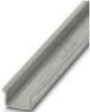
DIN rail, material: Steel, unperforated, 2.3 mm thick, height 15 mm, width 35 mm, length: 2 m
