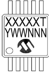
10-Lead MSOP (3x3 mm)
