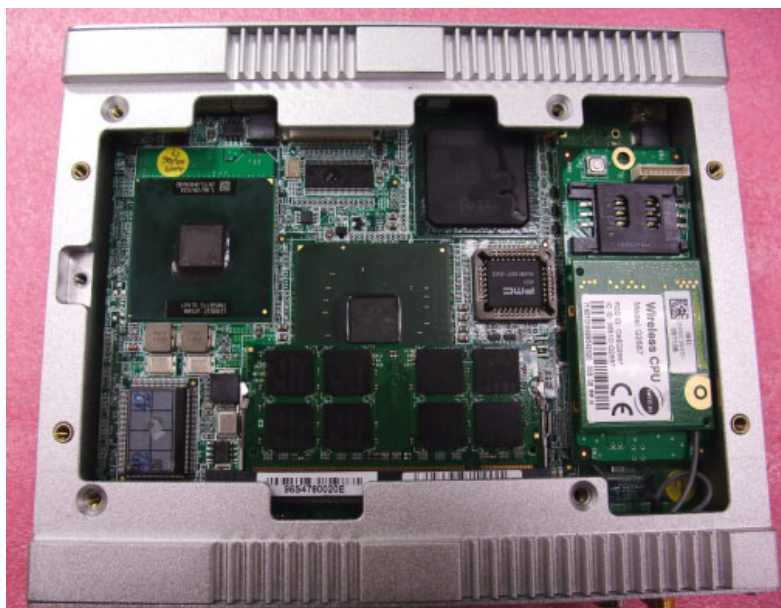
Figure 5.7 Installation AMO-EDGE on ARK-1388V
