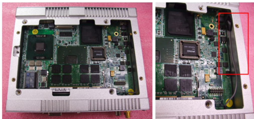
Figure 5.11 UMTS/HSDPA SMA cable internally
