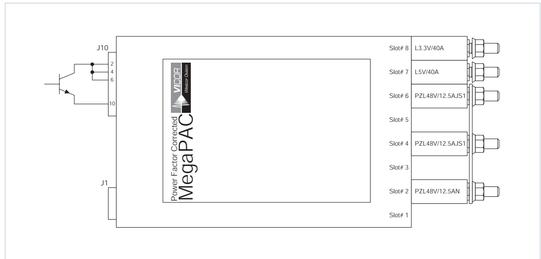
Figure 6 Enable / disable control of Maxi Arrays
