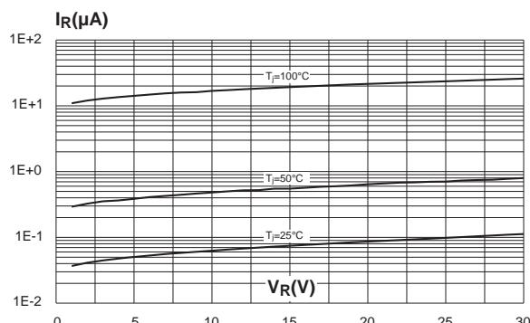
**Figure 4. Reverse leakage current versus junction temperature**
