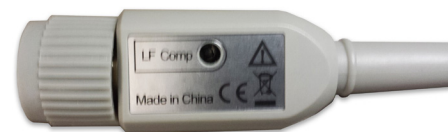
Figure 2. Low-frequency compensation adjustment (for N2840A/41A/42A/43A/53A)
