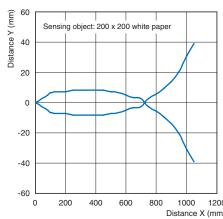
Size of Sensing Object vs. Sensing Distance
