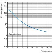
Excess Gain Ratio vs. Set Distance (Typical)
