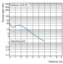
Excess Gain Ratio vs. Set Distance (Typical)
