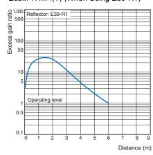
Excess Gain Ratio vs. Set Distance (Typical)
