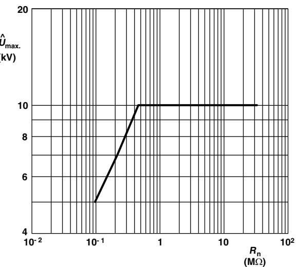
Maximum allowed peak pulse voltage in accordance with IEC 60065, 14.1.a); 50 discharges from a 1 nF capacitor charged to  $\hat{U}_{max}$ ; 12 discharges/minute (drift  $\Delta R/R \leq 2\%$ )
