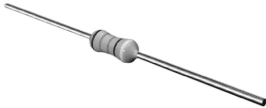
A metal glazed film is deposited on a high grade ceramic body. After a helical groove has been cut in the resistive layer, tinned electrolytic copper wires are welded to the end-caps. The resistors are coated with a light blue lacquer which provides electrical, mechanical, and climatic protection.
