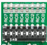
Figure 6-2: Tri-state DIP switch on PORTC
