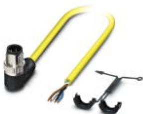
Sensor/Actuator cable, 4-position, PVC, yellow RAL 1021, Plug angled M12 SPEEDCON, A-coded, on free cable end, Cable length: 0.5 m
