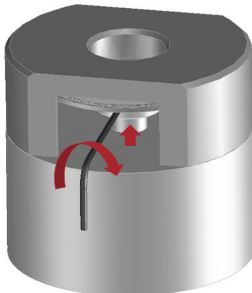
Figure 1d. Tighten the set screws
