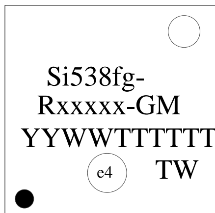
Figure 12.1. Si5381/82 Top Marking
