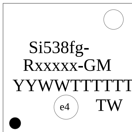
Figure 12.1. Si5381/82 Top Marking
