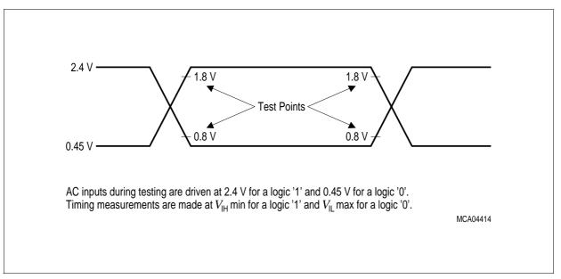
Figure 14 Input Output Waveforms
