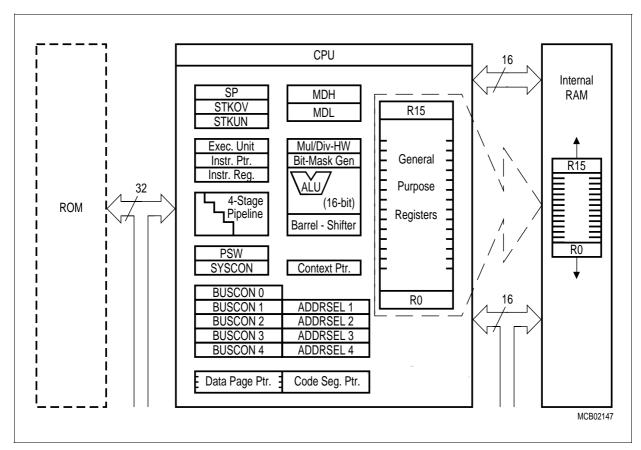
Figure 4 CPU Block Diagram
