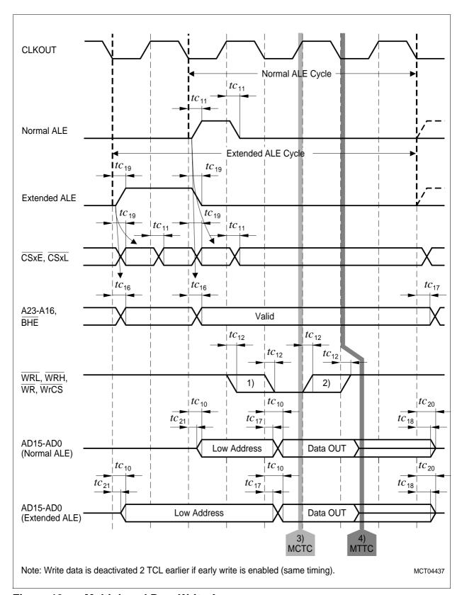
Figure 19 Multiplexed Bus, Write Access
