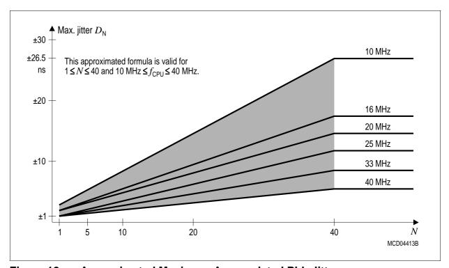
Figure 12 Approximated Maximum Accumulated PLL Jitter
