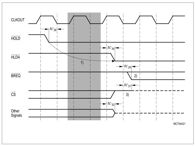
Figure 22 **External Bus Arbitration, Releasing the Bus**
