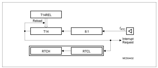
Figure 8 RTC Block Diagram
