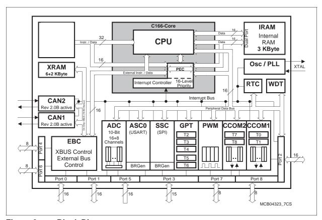
Figure 3 Block Diagram
