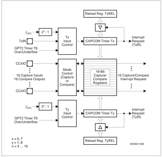
Figure 5 CAPCOM Unit Block Diagram
