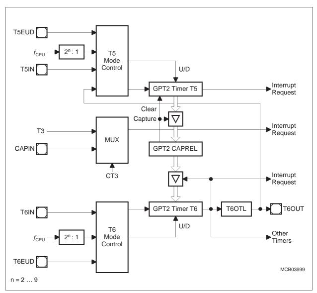
Figure 7 Block Diagram of GPT2
