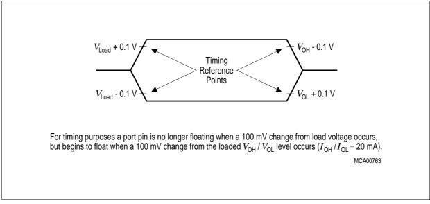
Figure 15 Float Waveforms
