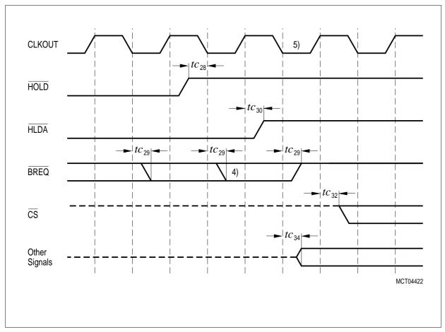
Figure 23 External Bus Arbitration, (Regaining the Bus)
