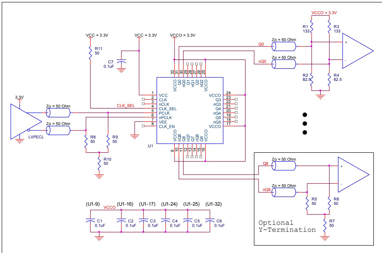
Figure 7. ICS853S031I Example LVPECL Clock Output Buffer Schematic
