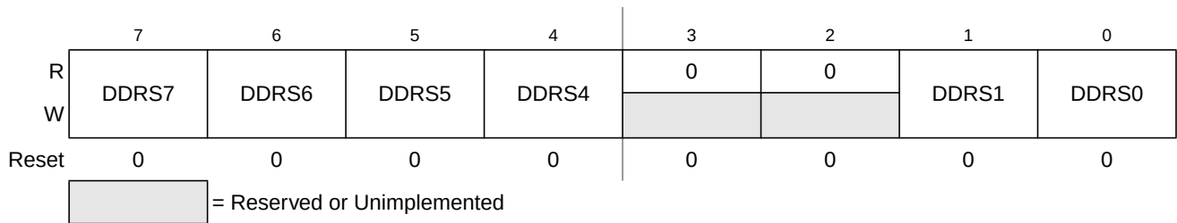
Figure 4-32. Port S Data Direction Register (DDRS)
