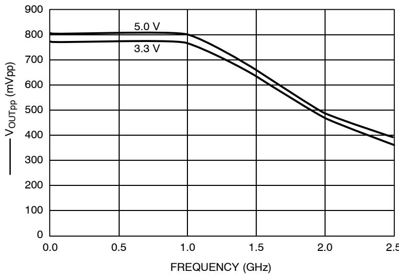
Figure 2. Typical  $V_{OUTPP}$  (mVpp) versus Frequency (GHz) @ 25°C
