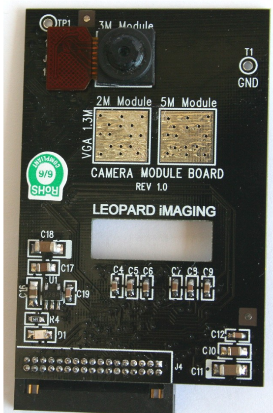
Figure 10. 3M Camera Board
