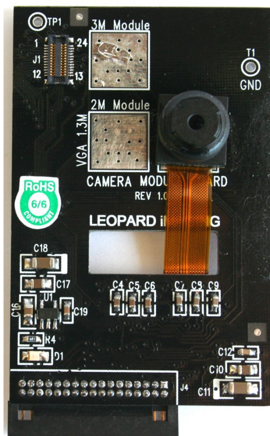
Figure 11. 5M Camera Board
