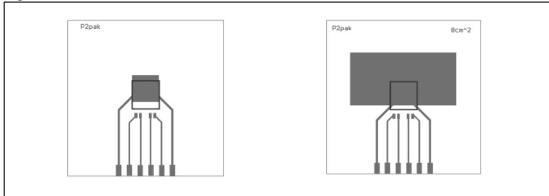
1. Layout condition of  $R_{th}$  and  $Z_{th}$  measurements (PCB FR4 area = 60 mm x 60 mm, PCB thickness = 2 mm, Cu thickness = 35  $\mu$ m, Copper areas: 0.97  $\text{cm}^2$ , 8  $\text{cm}^2$ ).
