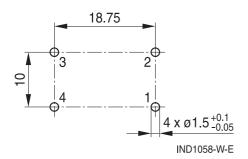
Tolerances to ISO 2768-cl / ISO 8015. Size ISO 14405 (E) All dimensions in mm
