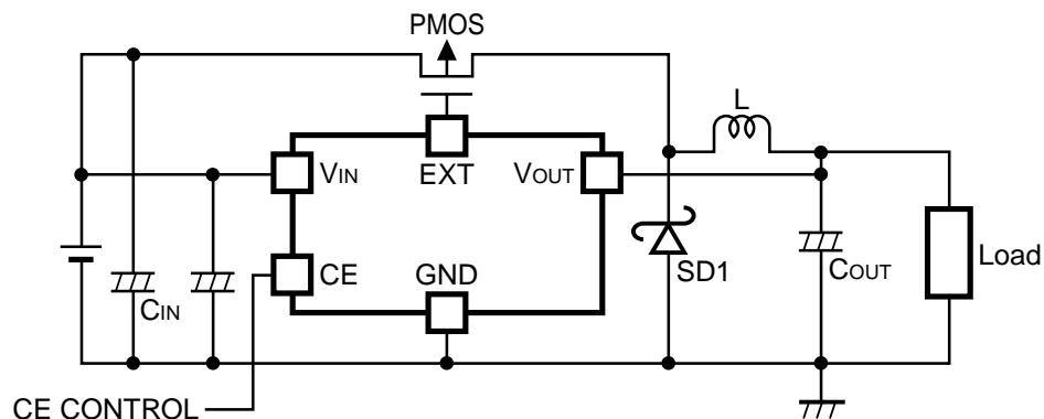
PMOS : HAT1020R (Hitachi), Si3443DV (Siliconix) L : CD105 (Sumida, 27 $\mu$ H)
