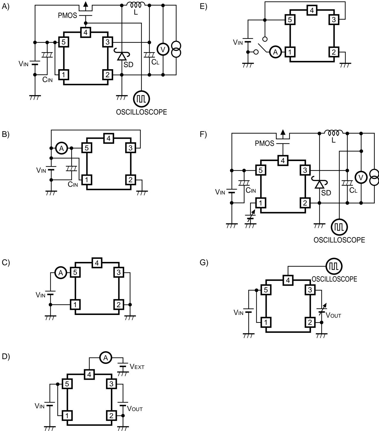
The typical characteristics were obtained by use of these test circuits.
