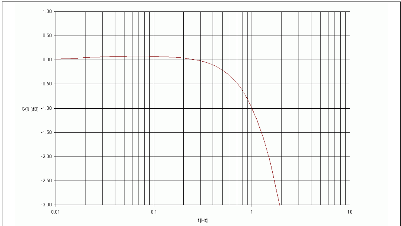
Figure 26 - Jitter Transfer Function - Detail
