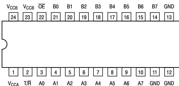
Figure 1. 24-Lead Pinout
