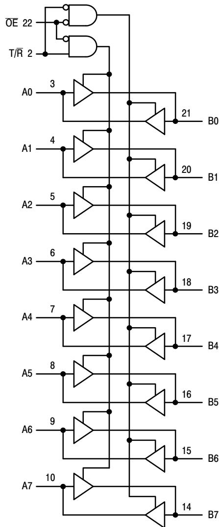
**Figure 2. Logic Diagram**
