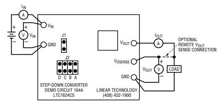
Figure 3. Proper Measurement Setup
