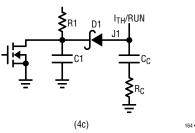
Figure 4. I<sub>TH</sub>/RUN Pin Interfacing
