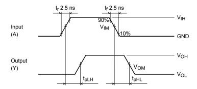
Figure 2 t<sub>pLH</sub>, t<sub>pHL</sub>
