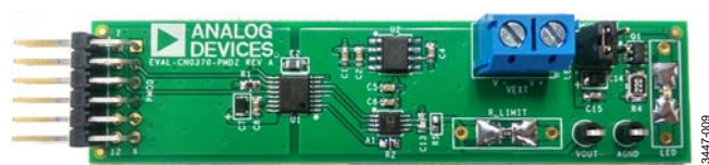
Figure 9. EVAL-CN0370-PMDZ Circuit Evaluation Board
