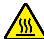
W3198 Heated/Hot Surface Hazard
