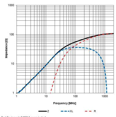
Test Equipment: E4991A or equivalent
