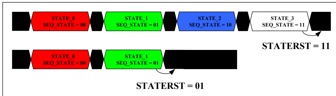
Figure 14 Setting the Sequence Length with STATERST
