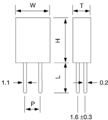
Figure 1) 190 ~ 249 KHz Front and Side Views
