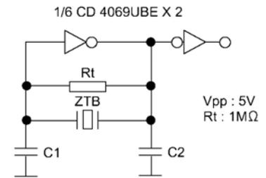
Figure 3) Test Circuit
