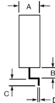
Figure 4) ZTBF (formed lead option) Land Pattern
