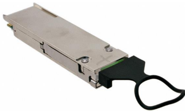
Figure 8-2 QSFP+ Loopback Fixture
