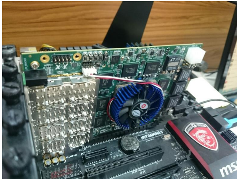
Figure 7-9 FPGA board installation on PC
