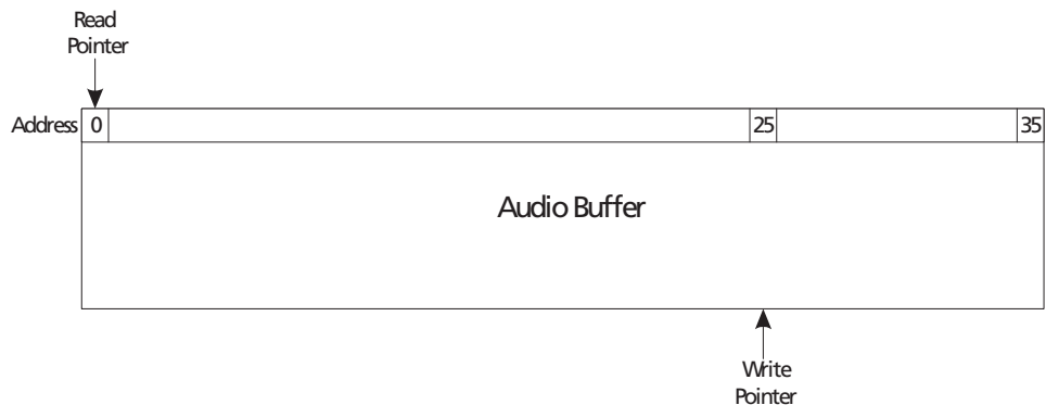
Figure 4-45: Audio Buffer After Initial 26 Sample Write
