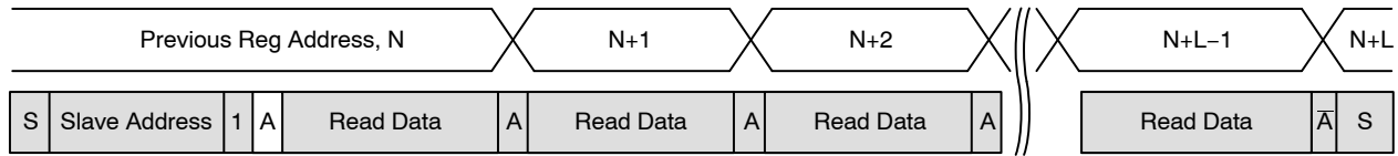
Figure 23. Sequential READ, Start from Current Location
