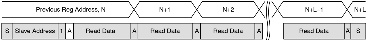
Figure 23. Sequential READ, Start from Current Location
