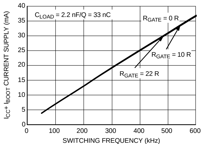
Figure 48. I_{CC1} Consumption vs. Switching Frequency with 33 nC Load on Each Driver @ V_{CC} = 15\text{ V}
