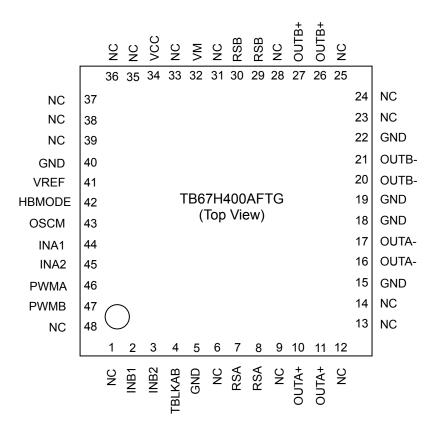
Note: Please connect the WQFN package corner pad and the exposed pad to the PCB ground pattern.
