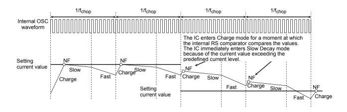
The Charge period starts as the internal oscillator clock starts counting. When the output current reaches the predefined current level, the internal RS comparator detects the predefined current level (NF); as a result, the IC enters Slow Decay mode.
