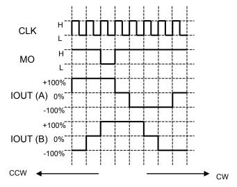
MO output shown in the timing chart is under the condition the MO pin is pulled up.
