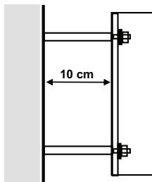
Data of power rating are referred to a resistor mounted vertically, with terminals in the lower side and away from the nearest surface at least 10cm, in order to avoid thermal influence from the wall.
