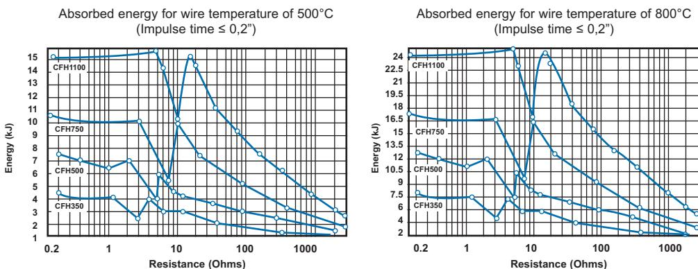
These graphs are irregular owing to the necessity to adapt the commercial dimension of wire to the resistance range, however they are enough to show the trend of this characteristic.
