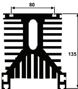
The distance between the axes of these two grooves is 80 mm. In this case both heat sink and resistor will be mounted upright. The length of the heat sink shall be at least 40 mm longer than the resistor's body (20 mm for each side).
