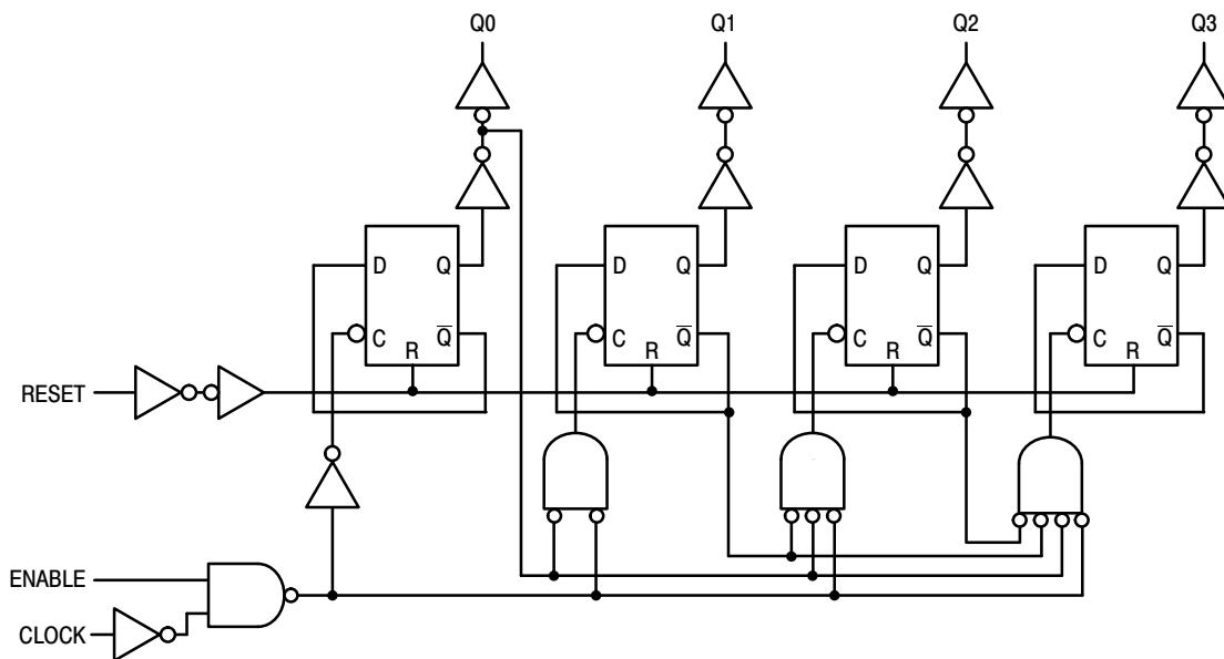
Figure 5. Binary Counter (MC14520B) Logic Diagram
