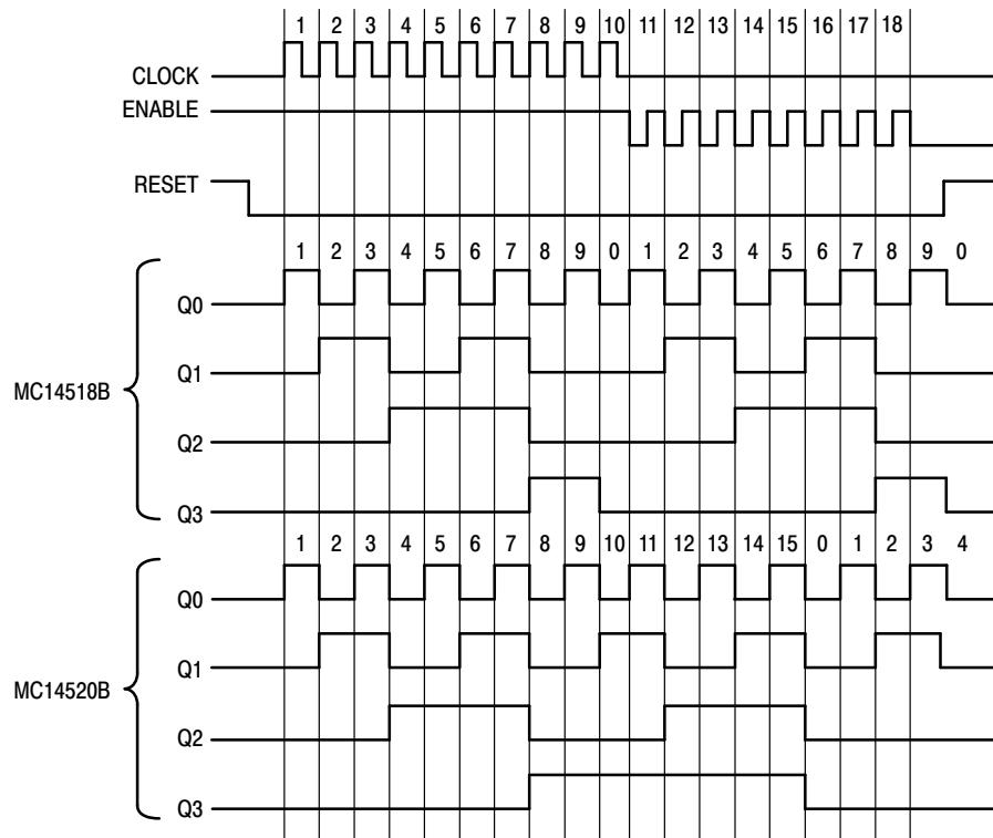
Figure 3. Timing Diagram
