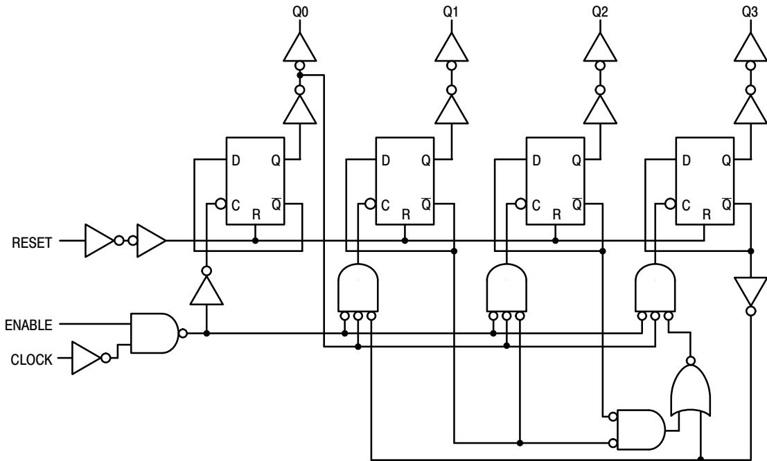
Figure 4. Decade Counter (MC14518B) Logic Diagram
