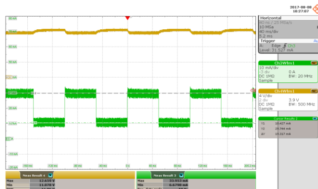
Figure 28 – 265 VAC, 0-100% Load Step. V_{MAX} : 12.343 V. V_{MIN} : 11.078 V. Upper: V_{OUT} , 4 V / div. Lower: I_{LOAD} , 10 mA / div., 40 ms / div.
