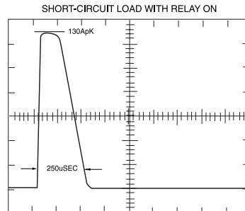
**SHORT-CIRCUIT LOAD WITH RELAY ON**
