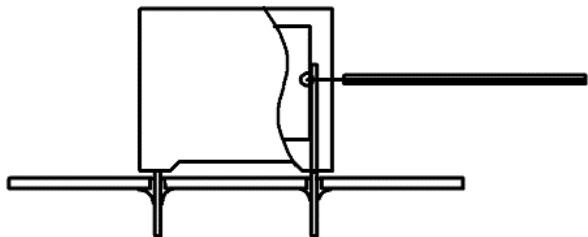
Temperature monitored inside the capacitor.
