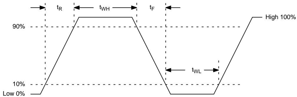
Figure 14. CCD Clock Waveform
