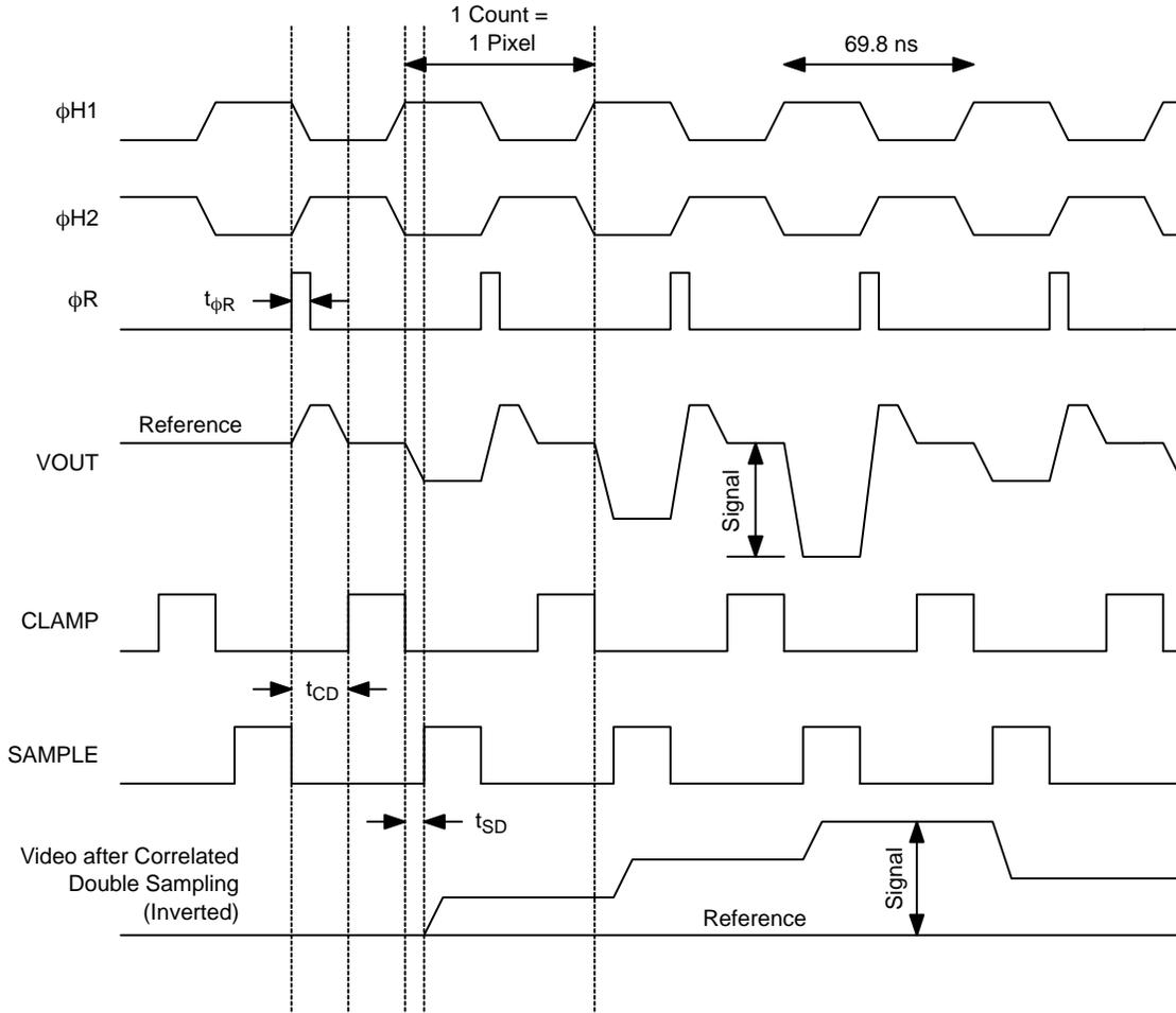
Figure 12. Pixel Timing
