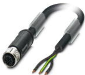
Power cable, 3-position, PVC, black, free cable end, on Socket straight M12 SPEEDCON, S-coded, Cable length: 1 m, For AC current up to 16 A/230 V
