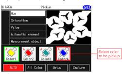
Specify the pickup area and press the Auto key to display 4 optional colors for pickup.
