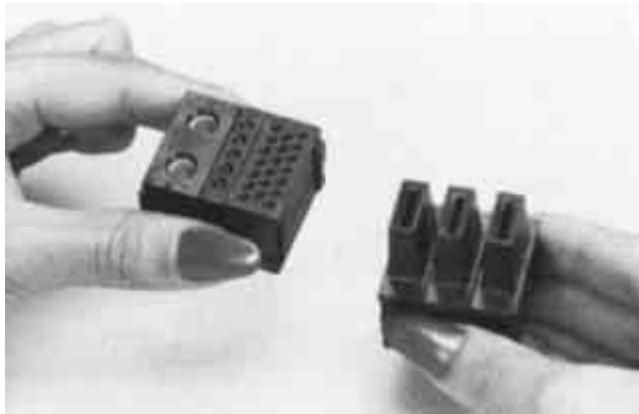
1. Align modules in desired order.
